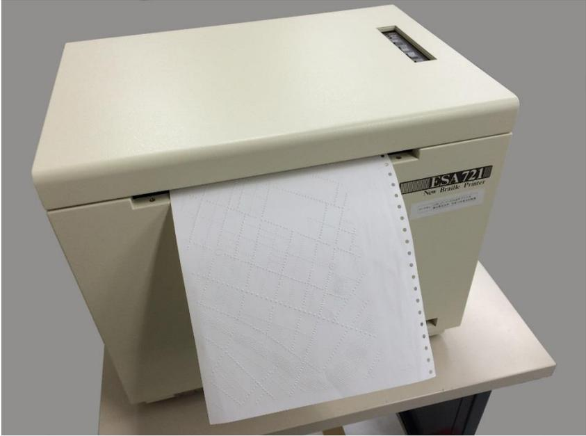
**Figure 2.3:** Braille Embosser for Producing Tactile Graphics
