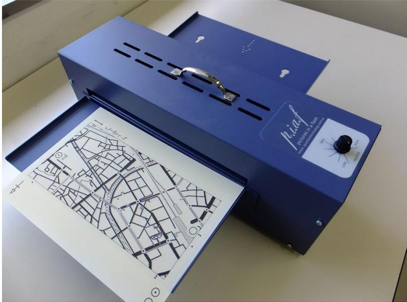
**Figure 2.2:** Swell-Form Graphics Machine for Producing Tactile Graphics
