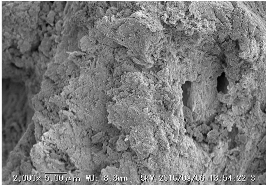
**Fig. 4.14:** SEM image of the CBC before fluoride adsorption
