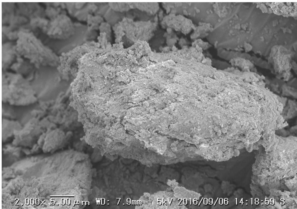
**Fig. 4.15:** SEM image of the CBC after fluoride adsorption
