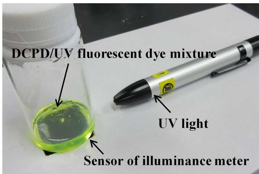
Fig.3-3 Setup for illuminance measure with UV irradiation.
