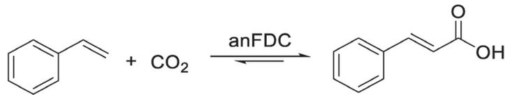
**Figure 1.** Schematic diagram of the carboxylation of styrene with prFMN dependent anFDC.
