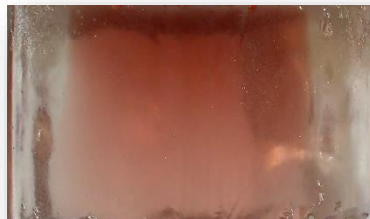
Fig. 3-13 Photo of as-grown reddish BGO crystal.
